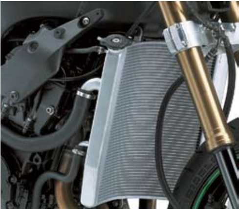
The radiator is narrower but taller than the previous unit to provide additional cooling capacity without adding aerodynamic frontal area. The water pump uses improved design borrowed from the ZX-14 to prevent cavitation during extended high-rpm use.
