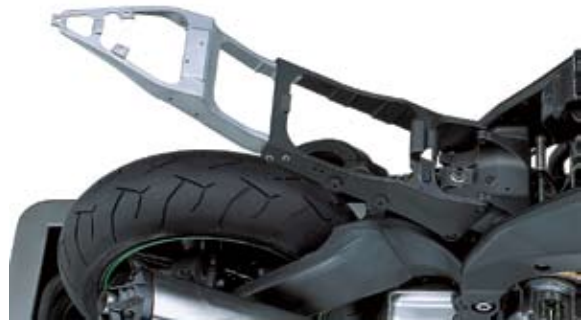
The rear subframe is now a two-piece aluminum die casting, with the rearmost section removable for racing purposes. The subframe now mounts directly to the main rear frame cross-member where the rear shock is mounted; Kawasaki claims that the more direct path to the rider improves feedback.
