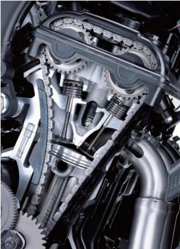
The new cylinder head features reshaped intake and exhaust ports, with all titanium valves (previously only intakes were titanium) and the exhaust poppets are now 1mm smaller. The combustion-chamber shape is revised, and the intake cams feature 0.6mm higher lift, while the exhaust cam timing has been retarded slightly for improved top-end power.
