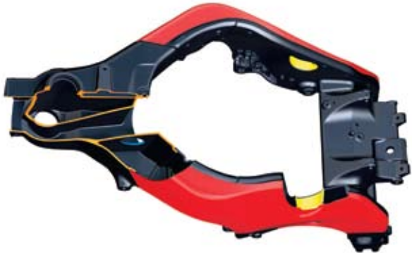
Changes to the new frame's rigidity were achieved by switching internal sections of the pressed main spar areas (red) from concave to convex shape, in addition to a tube welded into each spar (yellow) and additional strengthening ribs added to the top interior of the swingarm pivot plates. The steering-head pipe was moved forward 10mm and lengthened by 20mm for increased rigidity, while the ram-air intake was straightened and enlarged for better efficiency.
