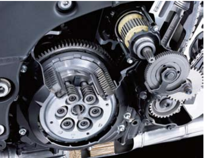
The same adjustable (via different spacers/springs) slipper clutch is kept for the new ZX-10R, while shorter first, fourth and fifth gear ratios—plus a lower final-drive ratio due to a one-tooth-larger rear sprocket—help retain midrange acceleration lost from the more aggressive cams. Crankshaft is 1kg lighter but maintains the same inertia due to reshaped counterweights.
