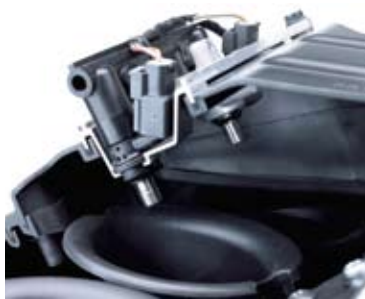
Throttle bodies now feature oval subthrottle plate sections for improved throttle response, and the ZX-10R finally gets secondary shower-style injectors this year for better top-end power. A straighter and larger ram-air intake tract combines with an airbox twice as large (from four- to eight-liter capacity, made possible by a flat-type fuel pump) to enhance volumetric efficiency.
