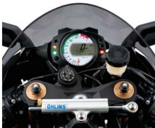
The new instrument panel has a UV-blocking glass to make the LCD display brighter, and the tachometer numbers are labeled better. An adjustable Öhlins steering damper helps quell headshake tendencies.
