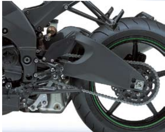
Constructed from pressed-aluminum-sheet beams welded to a die-cast pivot/shock-mount section, the ZX-10R's swingarm is now braced on top instead of the bottom, presumably to make room for the under-engine exhaust. The swingarm pivot was lowered 2mm.
