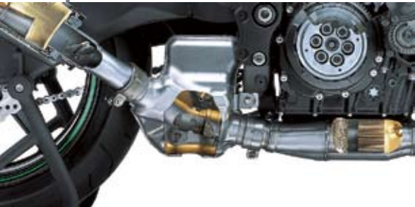
Freer-flowing catalyzers in both primary and secondary collectors clean up the Kawasaki's exhaust enough to pass EPA and Euro III emissions standards, while the pre-chamber and exhaust valve help quell noise.
