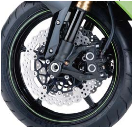
The radial-mount brake calipers now use two brake pads instead of four for less aggressive response, with different-size leading/trailing pistons to maintain even pad wear. The petal-type discs grow to 310mm from 300mm while becoming 0.5mm thinner. Disc carriers are now aluminum, with three more buttons per disc to spread load and heat better.
